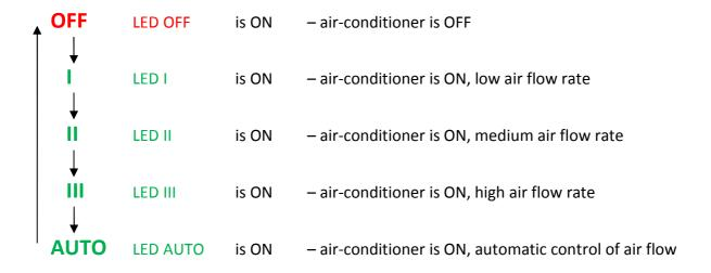
Note: there is always only one LED lighting in this column, remaining LEDs will be OFF.
